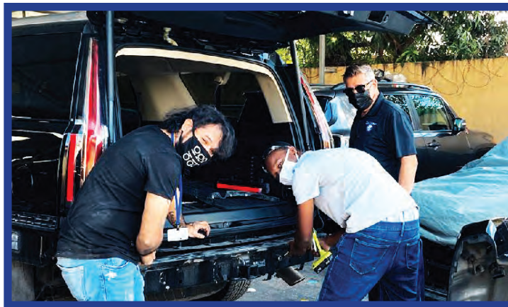
► Above Mr. Henry Gonzalez, Owner of De Colores Providing LHTC Students the Technical Knowledge on How to Remove the Hitch Components on a Vehicle, Once the Bumper was Removed
